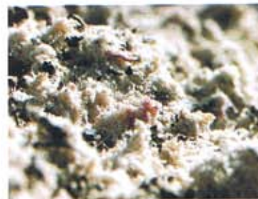
A new surface called Polytrack made its debut at the racetrack. The material is a combination of polypropylene fibers, recycled rubber and silica sand with a wax coating.
